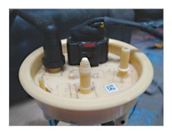
Remove the blanking nipple from the end of the spare fuel spigot on the sender unit.
