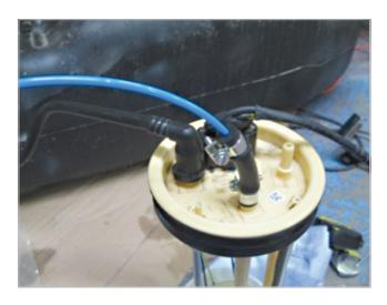
Pass the straightened 230mm, 4 x 1mm Ø fuel tube through the hole into the fuel tank until the 7.5/3.5mm Ø rubber adaptor is over the spigot .
