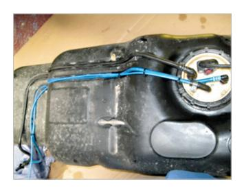
6. Route the remaining 4 x 1mm  $\emptyset$  fuel tube to the FM pump mounted at 15-35° angle in the normal manner.
