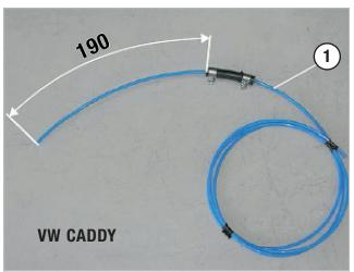
1. Warm the fuel tube 4 x 1mm Ø on a length of approx. 250mm with a hot-air heat gun to straighten pipe to manufacture.
