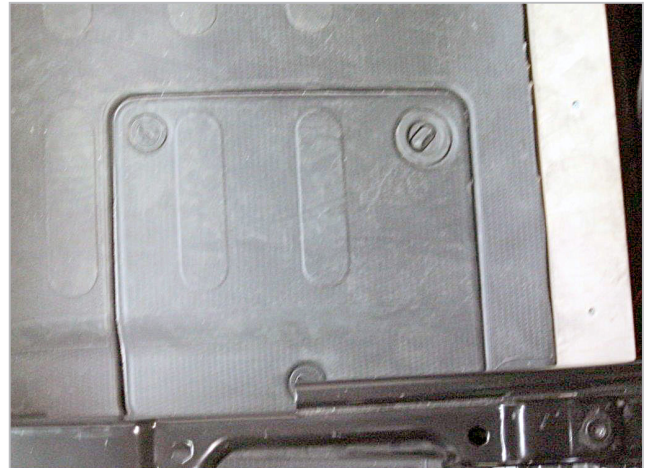
2. Remove both fuel sender access covers on cab floor.
