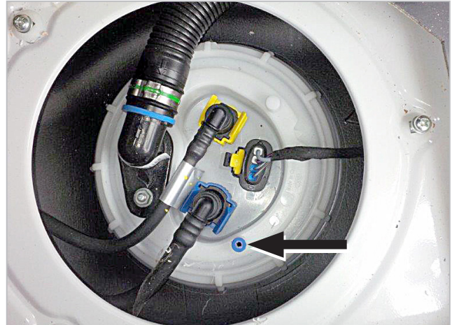
4. Drill hole out to 4.2mm. Avoid swarf entering fuel tank.
