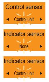
Select by turning the operating button and confirm by pressing.
