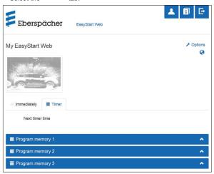
The timer function can be used for air and water heaters. Each program memory can be used for heating or ventilation and can be set accordingly.
